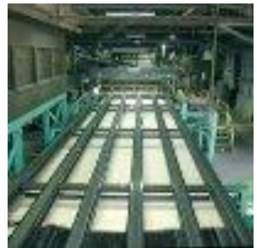
Tray system between Coe lathe and Durand-Raute clipper, with Ventek scanner at the end of the line.
